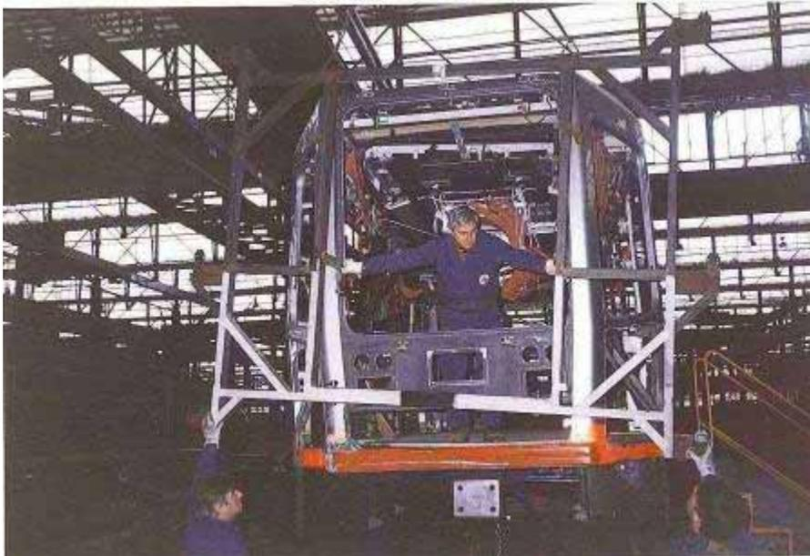
**Figure No. 2 – LRV No. 1407 being aligned using an alignment fixture**
